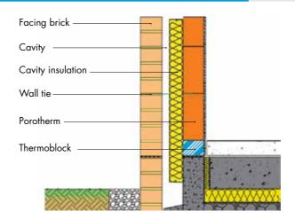
Specification: The cellular clay block (e.g. Porotherm T8) is fixed onto the Thermoblock with 12mm bricklayers mortar (min. mean compressive strength of 25 N/mm<sup>2</sup>). The cellular clay brick wall is laid directly on top of the Thermoblock if the combined dead and imposed load is <2N/ mm<sup>2</sup>. For loads in excess of 2N/mm<sup>2</sup>, an aircrete block is laid on the Thermoblock to form the starter course of the cellular clay block wall.
