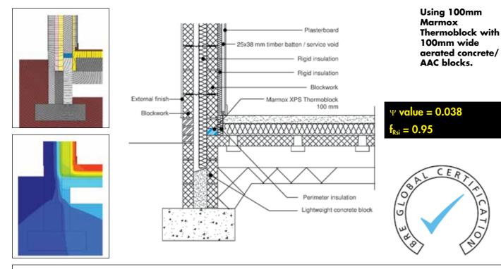
Typical Specification: A single course of Marmox Thermoblock: 600mm(l) x 100/140/215mm(w) x 65mm(ht) is the starter course for the inner leaf of the wall in place of the bottom row of blocks. Thermoblock is fixed to the floor with normal mortar which is also used to lay subsequent courses of bricks/blocks on top. If using lightweight blocks, this initial layer of mortar should be 15mm.
