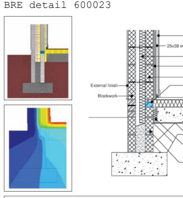
Typical Specification: A single course of Marmox Thermoblock: 600mm(l) x 100/140/215mm(w) x 65mm(ht) is the starter course for the inner leaf of the wall in place of the bottom row of blocks. Thermoblock is fixed to the floor with normal mortar which is also used to lay subsequent courses of bricks/blocks on top. If using lightweight blocks, this initial layer of mortar should be 15mm.
