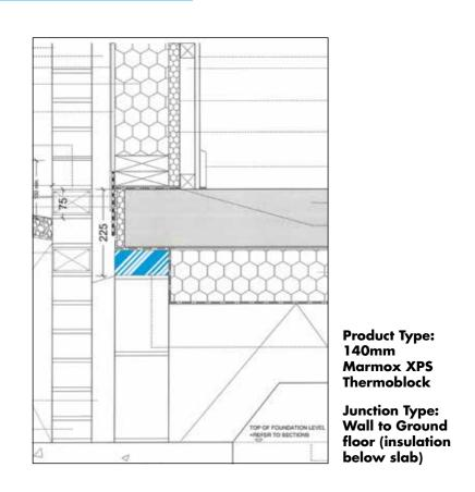
**Specification:** A single course of Marmox Thermoblock:  $600mm(l) \times 100/140/215mm(w) \times 65mm(ht)$  is fixed using normal mortar on to top of the foundation blocks (inner leaf) directly underneath the load bearing concrete slab on which the timber frame is fixed.
