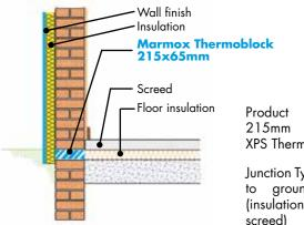
Type: 215mm Marmox XPS Thermoblock Junction Type: Wall to ground floor (insulation below
